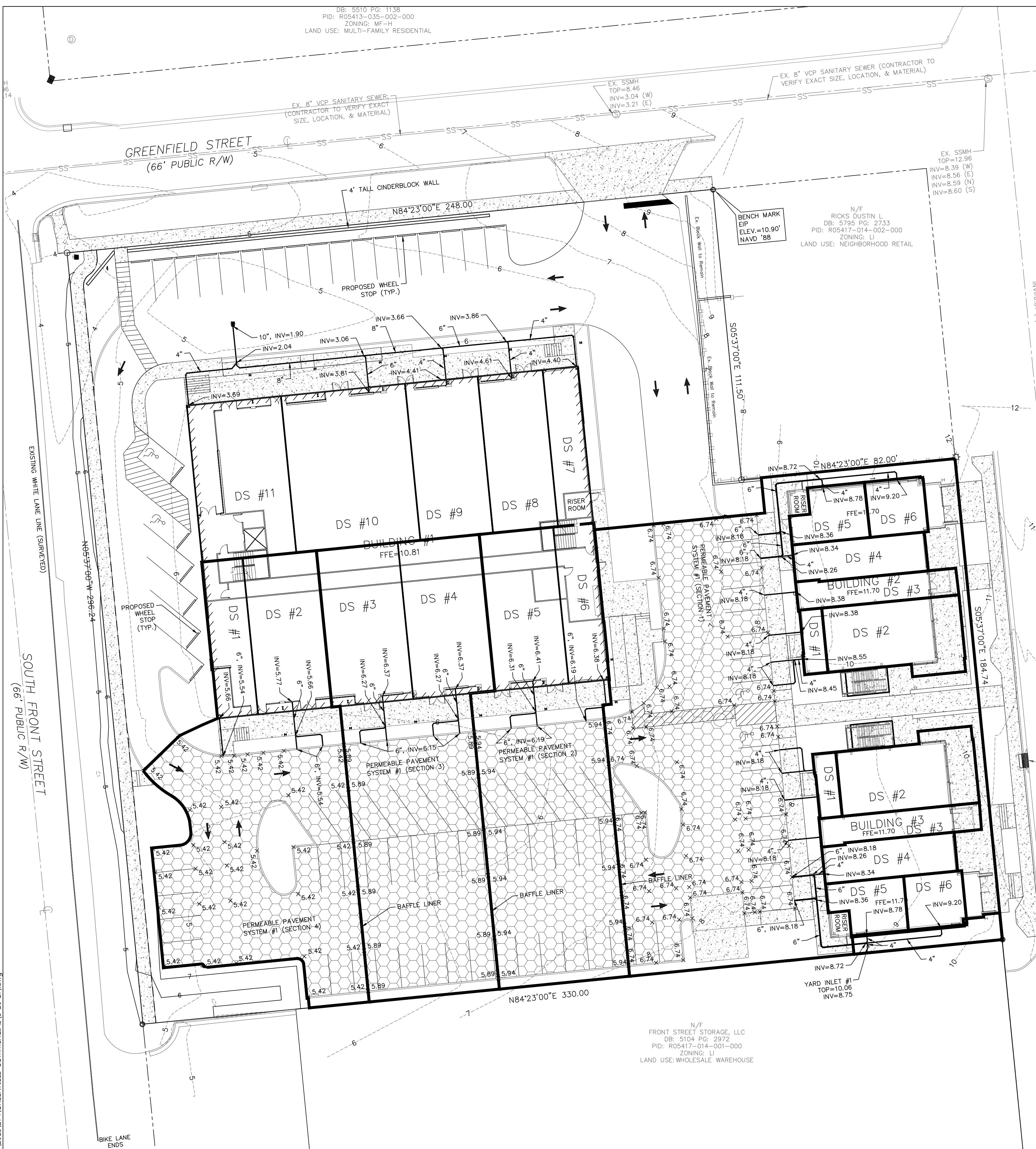
ROOF DOWNSPOUT PIPING (LAYOUT & DRAINAGE AREA MAP) & PERMEABLE PAVEMENT SUBGRADE GRADING PLAN SCALE: 1"=20'
